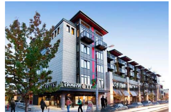
Variation In Architectural Projection, Using Color And Lighting Can Break Roof Form And Line In The Facade.
